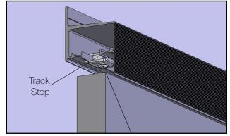
Install End Caps. Install Endcaps, one left and one right, by simply press fitting to either end of the track. End Cap
