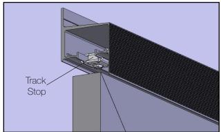
Install End Caps. Install Endcaps, one left and one right, by simply press fitting to either end of the track.
