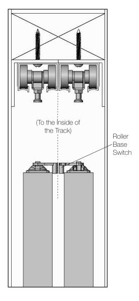
Attach Roller Wheels to Doors. Lift the Door to the Track (NOT SHOWN) and Insert Roller Wheel Stud into Roller Base. Close Roller Base Switch by moving from left to right. A tight snap should be felt and heard.
