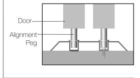
\*Installing Contractor/Personnel is responsible for providing secure Mounting Frame/Structure in which to install track. Open | Close Doors is not liable for the installation of door/track systems installed with insufficient Mounting Structures.
